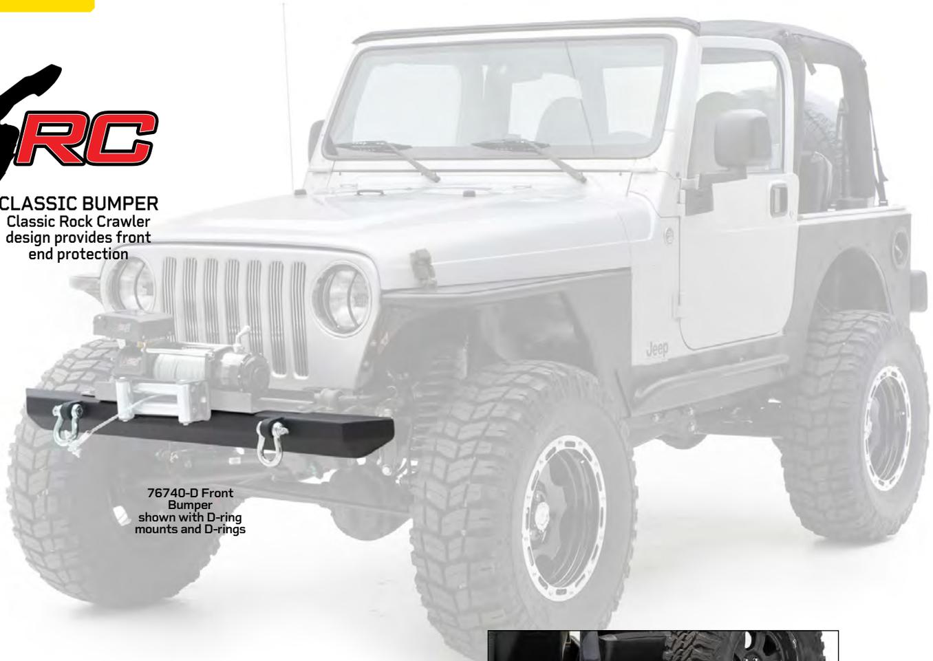
76740-D Front Bumper shown with D-ring mounts and D-rings
