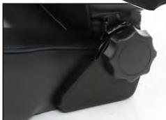
[ C.-D.] Reclining knobs on both sides of seat allows seat to function on either side
