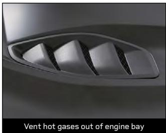
Vent hot gases out of engine bay
